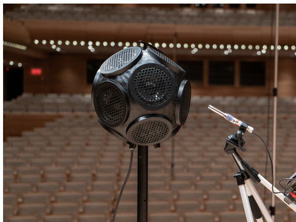
(a) Loudspeaker with one of the calibrated microphones used during measurements at the Maison Symphonique.
